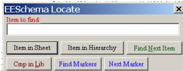
You can search a component, a value, or a text string in the current sheet or in the whole hierarchy. The cursor will be positioned on the found element, in the concerned sub-sheet.
